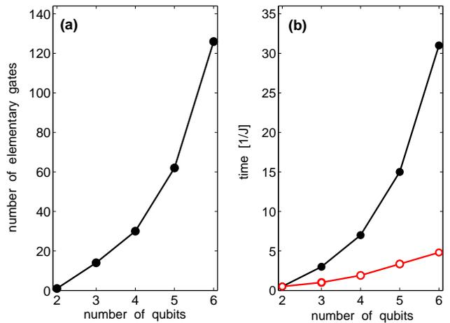
FIG. 4: (a) Network complexity of the  $C^{n-1}$ NOT-gate on complete coupling topologies  $K_n$  [41]. (b) Time complexity of the  $C^{n-1}$ NOT-gate on complete coupling topologies. Upper trace: analytical times for decomposition into standard gates ( $\bullet$ ) [41]. Lower trace: speed-up by time-optimal control with shortest times ( $\circ$ ) currently needed for realising  $C^{n-1}$ NOT by numerical control rounded to  $0.01 J^{-1}$ .
