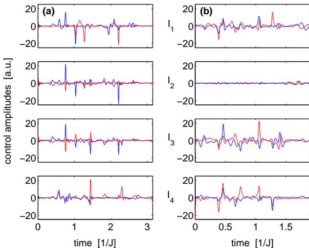
FIG. 5: Time course of controls for the shortest realisations obtained for the following quantum modules: (a) the QFT on a linear coupled four-qubit system ( $L_4$ ); (b) the  $C^3\text{NOT}$ -gate on a fully coupled four-qubit system  $K_4$ . Traces in blue: amplitudes for  $\sigma_{\ell x}$ -controls ( $x$ -pulses); red: amplitudes for  $\sigma_{\ell y}$ -controls ( $y$ -pulses) on the spins  $\ell = 1, 2, 3, 4$ .
